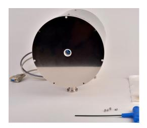
Remove the loose white thermal insulation. Be sure to get the two annular rings of thermal insulation around the can. Leave the black plastic insulation stop in place to keep the insulation around the tube from falling into the can while loading the cavity.
