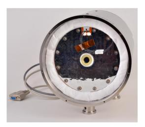
Disconnect the front heater (there will be a white connector that attaches the flange heater to the body). Unscrew (with a 3 mm metric Allen T wrench) and remove the vacuum chamber flange, taking particular care to hold the flange while the last screw is removed so it doesn't scratch the sealing surface while moving against the can. Place the flange O-ring side up on a clean cleanroom wipe, taking care not to damage the window.
