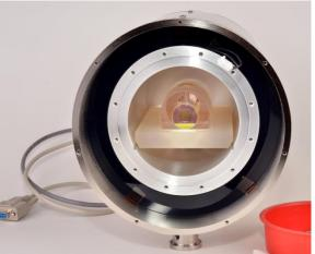
Replace the vacuum end flange, and fasten the screws in a diametric pattern (that is, a pattern that would follow the points of a clock, first 12 o'clock, then 6 o'clock, 3 o'clock, then 9 o'clock, and repeat this diametric pattern for the two other sets of four bolts. Repeat tightening three or four times until all the bolts are secure, using only moderate torque on each bolt.
