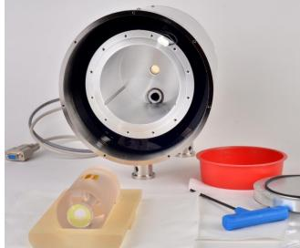
Load the Zerodur mounting block into the can by sliding the block into the grooves in the chamber. Try to align the block so that there is an equal gap on each side with respect to the vacuum chamber.
