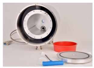
Load the cavity onto the Zerodur mounting block, using the Viton balls provided. Place the 4 viton balls in the machined holes in the mounting block. Center the cavity in the cutout and lower it into the support. Remove the kapton tape covering the vent hole prior to loading the cavity.
