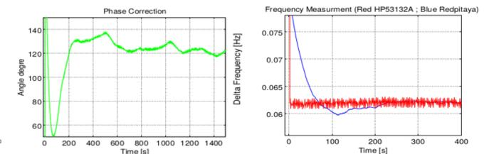
For the sake of reconfigurability demonstration and ease development, we present here simple tests on medium quality quartz oscillator while data analysis is performed through the embedded CPU unit. Concurrent RAM transfer and calculations benefits from multithreaded techniques.
